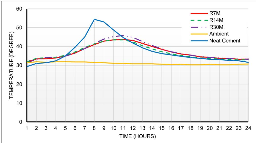
Figure 4. Hydration rate of 0% using different fibre length
