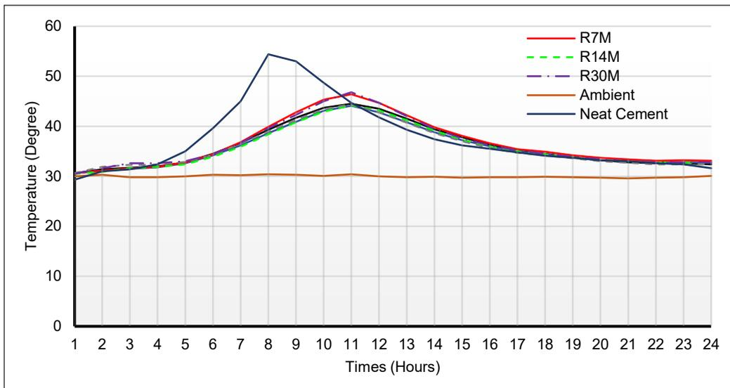
Figure 5. Hydration rate of 0.4% using different fibre length
